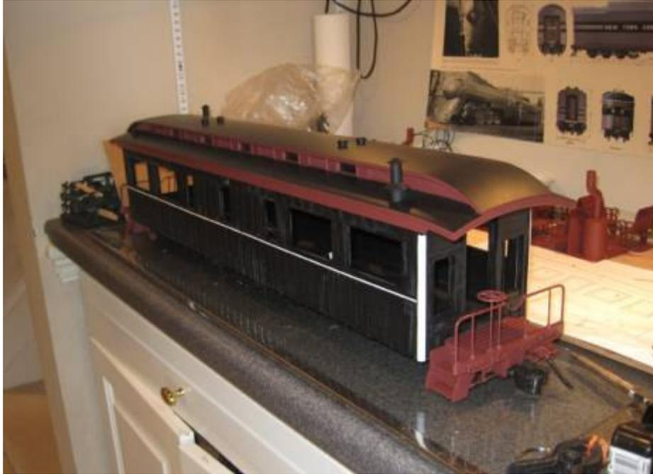
Starting to look like a coach! This is a test fit on the underframe - still to be done are the railings and interior. This would be a good time to add the tabs to attach the roof to the sides, and the sides to the floor (See General Info Notes.)
