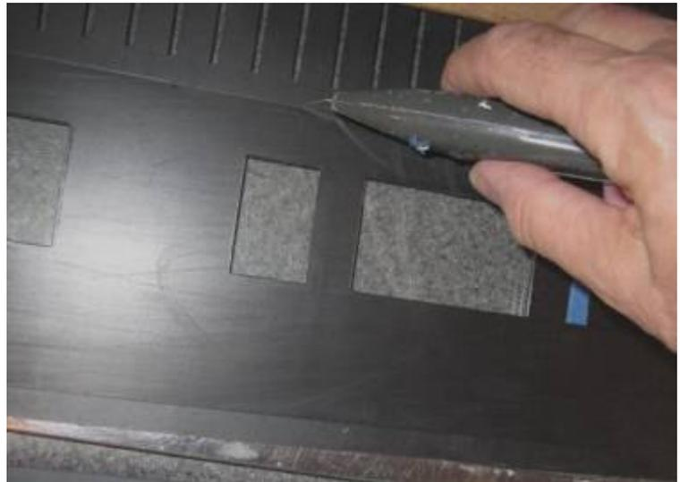
If you lightly score the ends of the battens, you can then lift the sides and put them safely away while you finish the cut using a metal straight edge.
