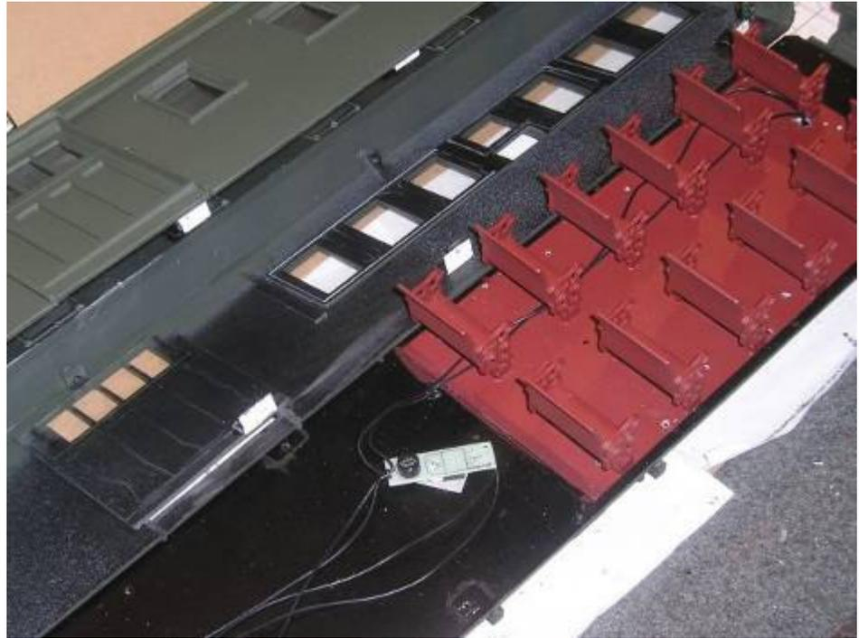
The seats are difficult to remove from their plastic sub-floor; they are firmly glued in place. If you want to change the spacing, I
