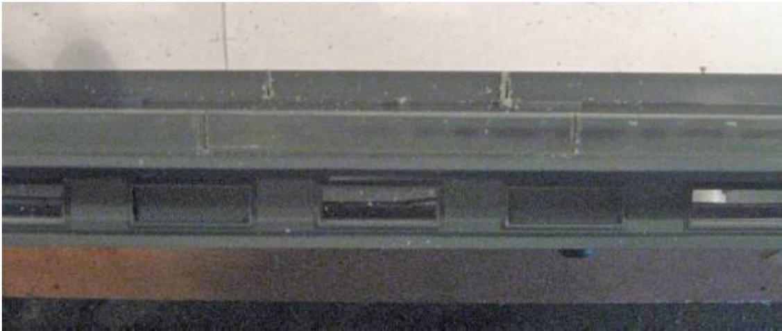
Cut the letterboard down to the roof but no more with a small saw. Make it slightly smaller than marked - you can always widen it but it won't be easy to make it narrower. I snapped out the strip by scoring along the edge of the roof with a sharp knife, and then I gripped the end in pliers and carefully bent it until it started to break. Repeat at the other end and the strip will pop out. File the rough bits down and check the fit.
